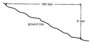
Figure 3. Diagram showing a 5 percent slope.
