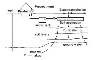
Figure 6. Soil Disposal of Septic Tank Effluent.
